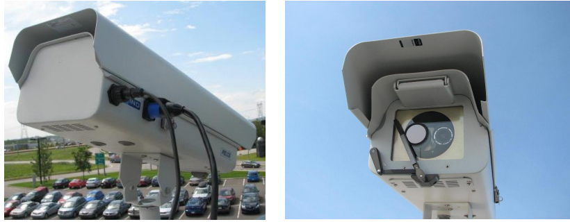
Fig. 3. LWIR / colour acquisition platform developed at INO.
